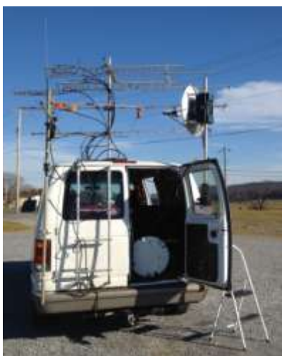
The 24 GHz QSO between rover K1DS and fixed-station K3TUF was made with the dish on the floor of the van as seen here. Due to winds, Rick K1DS couldn’t climb atop the van to mount the dish but reports solid 5-9 signals anyway!! (Photo by K1DS)
