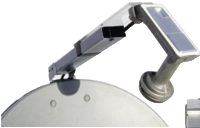
Figure 11 — Aiming the RT at the Sun, note LNB shadow location.
