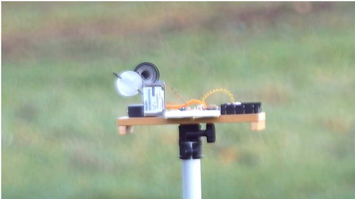
Figure 27. The transmitter observed through Celestron FirstScope with a video camera - distance 109m
