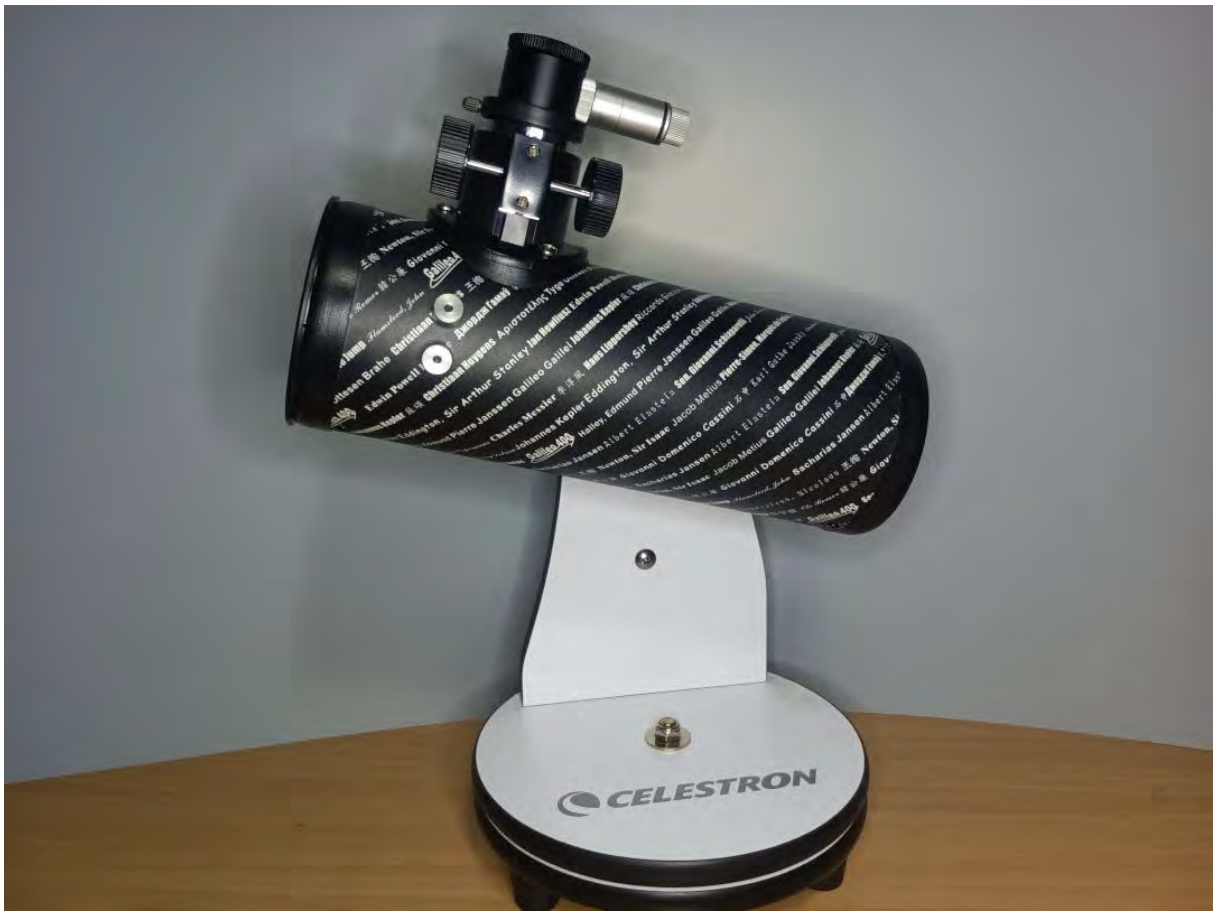
Figure 18. Celestron FirstScope: Newtonian reflector, mirror diameter 76mm, FL 300mm
