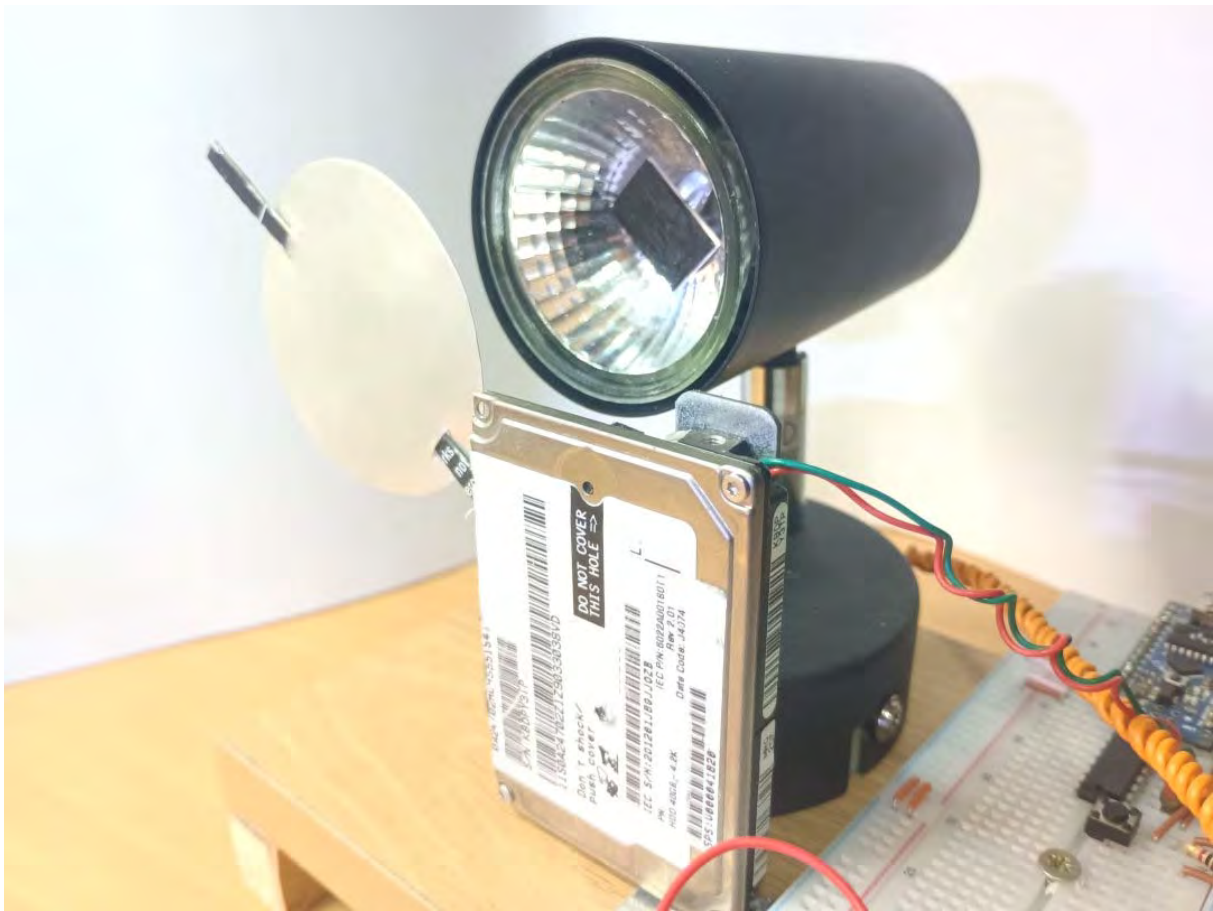
Figure 12. Heater assembly with paddle mechanical modulator
