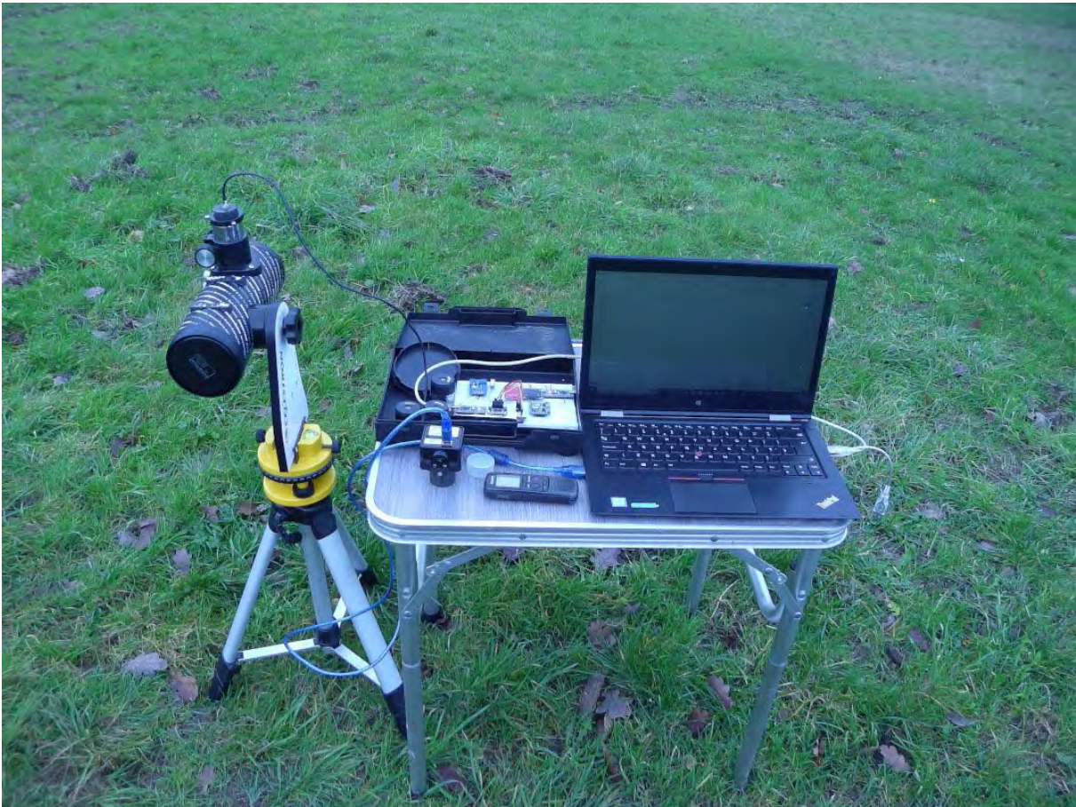
Figure 24. Geodesic Tripod with receiver
