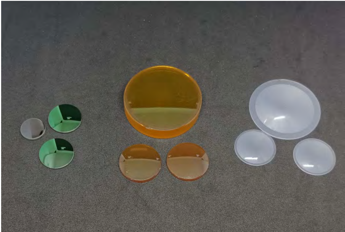
Figure 6. Lenses for the 30THz band. From left Germanium, Zinc selenide, High-density polyethylene (HDPE)
