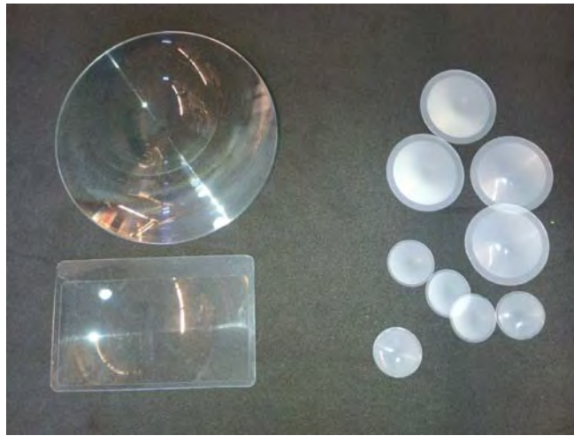
Figure 7. Visible light Fresnel lenses (PMMA), opaque for 30THz (left), and Thermal Fresnel lenses (HDPE), transparent for 30THz (right)
