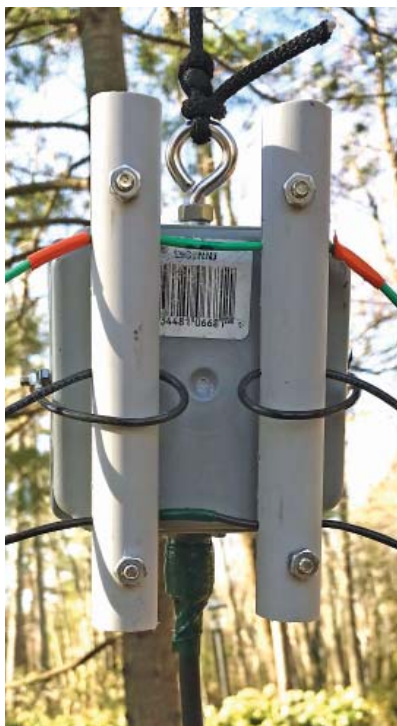
Figure 4 — The back of the feed-point box shows the center-driven wire and coupled-resonator wires above (for 10 meters) and below (for 20 meters). The orange tape on the 10-meter wire is for restricting movement through the spacer.
