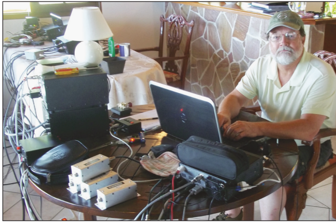
Here is Jeff, FJ/K5WE, chipping away at the pileup. Notice the group of band-pass filters on the table; these allowed the two stations to be on the air simultaneously and still play nice with each other.
