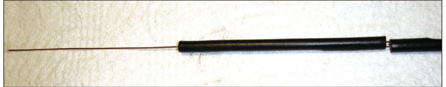
Figure 7 — Top section of the antenna with the 4 1/2 inch exposed center conductor acting as a vertical element.
