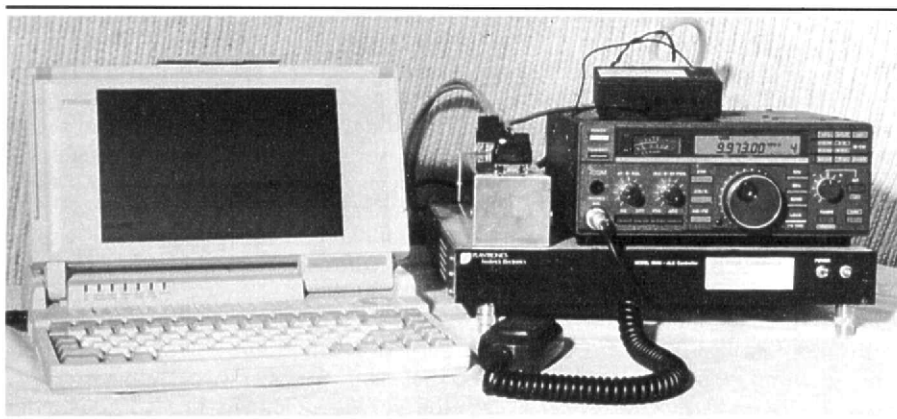
Fig 1—Low-cost HF ALE radio system.
